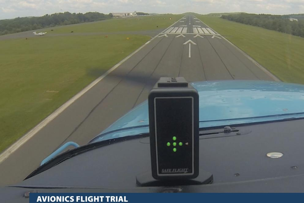
*The latest generation SafeFlight SCc has a glareshield-mounted digital speed indexer with Geiger counter—like audio output. The display in the photo to the left indicates an on-speed condition for landing.*
