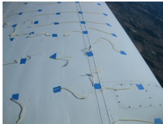
A tufted wing in near-stall, leading edge to the right
